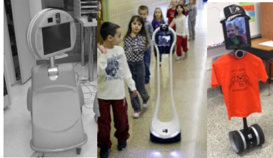
Figure 4.1. From left to right, PEBBLES, VGo, and Double Robots used in schools
