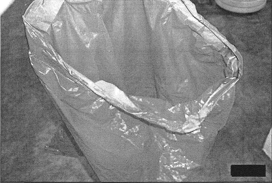
Figure A-3. The edge of the bag opening is wrapped around the wire frame and taped to it.
