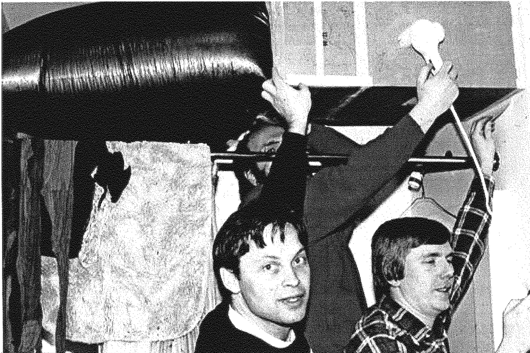
Figure A-5. Exhaust measurement using a hairdryer and cardboard box (Building Science Corp)
