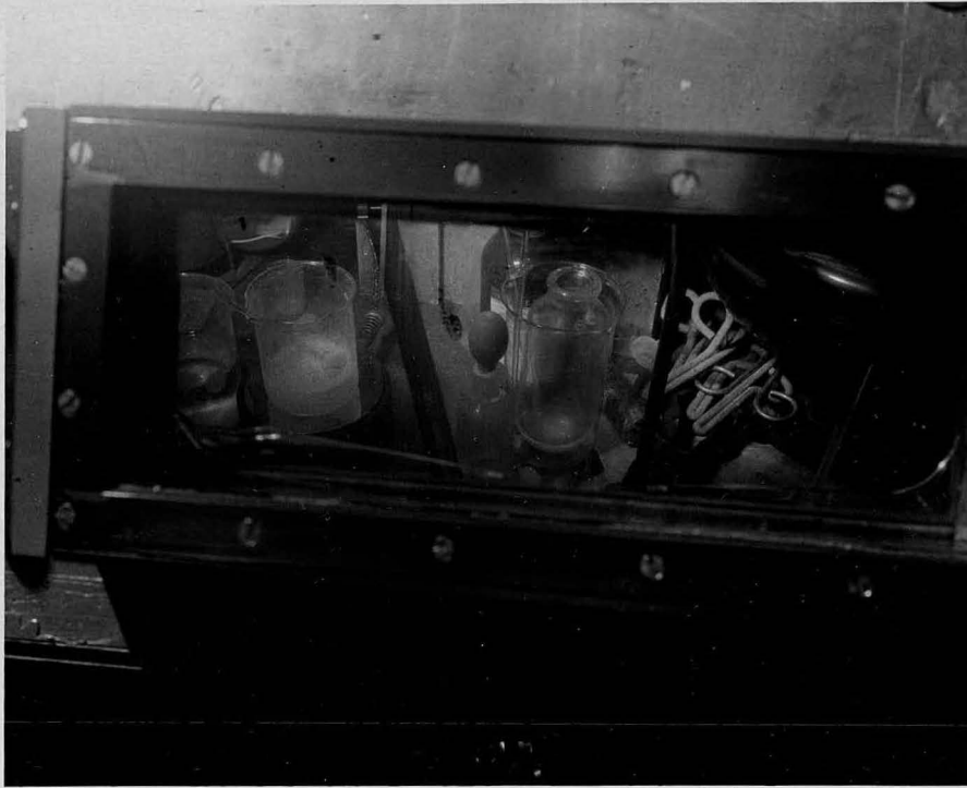
FIG. 17 VIEW THROUGH 3 INCH LEAD GLASS AND LEAD SHIELDED BERKELEY BOX
