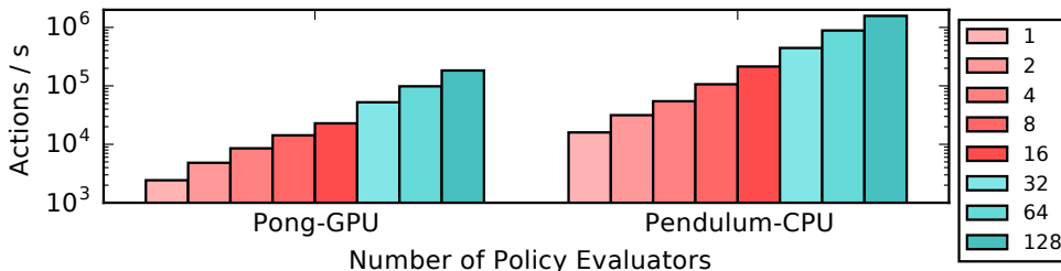
Figure 3.7: Policy evaluation throughput scales nearly linearly from 1 to 128 cores. PongNoFrameskip-v4 on GPU scales from 2.4k to ~200k actions/s, and Pendulum-v0 on CPU from 15k to 1.5M actions/s. We use a single p3.16xl AWS instance to evaluate from 1-16 cores, and a cluster of four p3.16xl instances from 32-128 cores, spreading actors evenly across the cluster. Rollout workers (evaluators) compute actions for 64 agents at a time, and share the GPUs on the machine.
