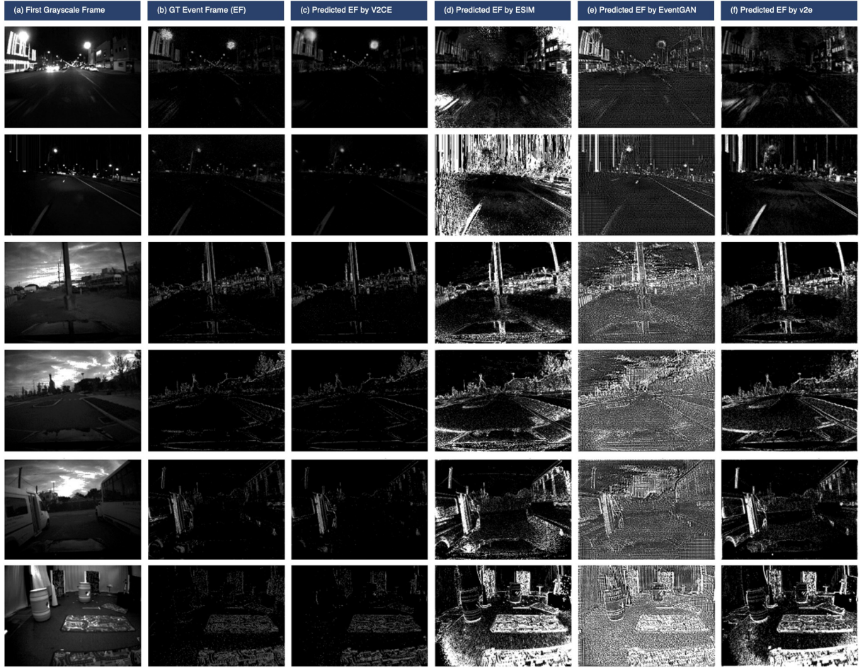
Figure 2.4. Event frame comparison between V2CE and baseline methods. Event frames are clipped to the maximum value of their corresponding ground truth event frames and then normalized.
