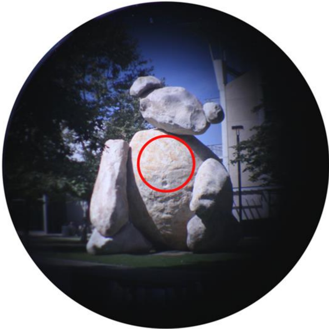
Figure 2-6: Image of the Stone Bear on UCSD campus. The object is approximately 25 meters from the optomechanical eye model. The darkening around the edges is caused by the limitation of the numerical aperture of the fiber and its inability to couple light efficiently at high fields of view, similar to the Stiles-Crawford effect. The red circular area represents the equivalent of the macular region in human eye.
