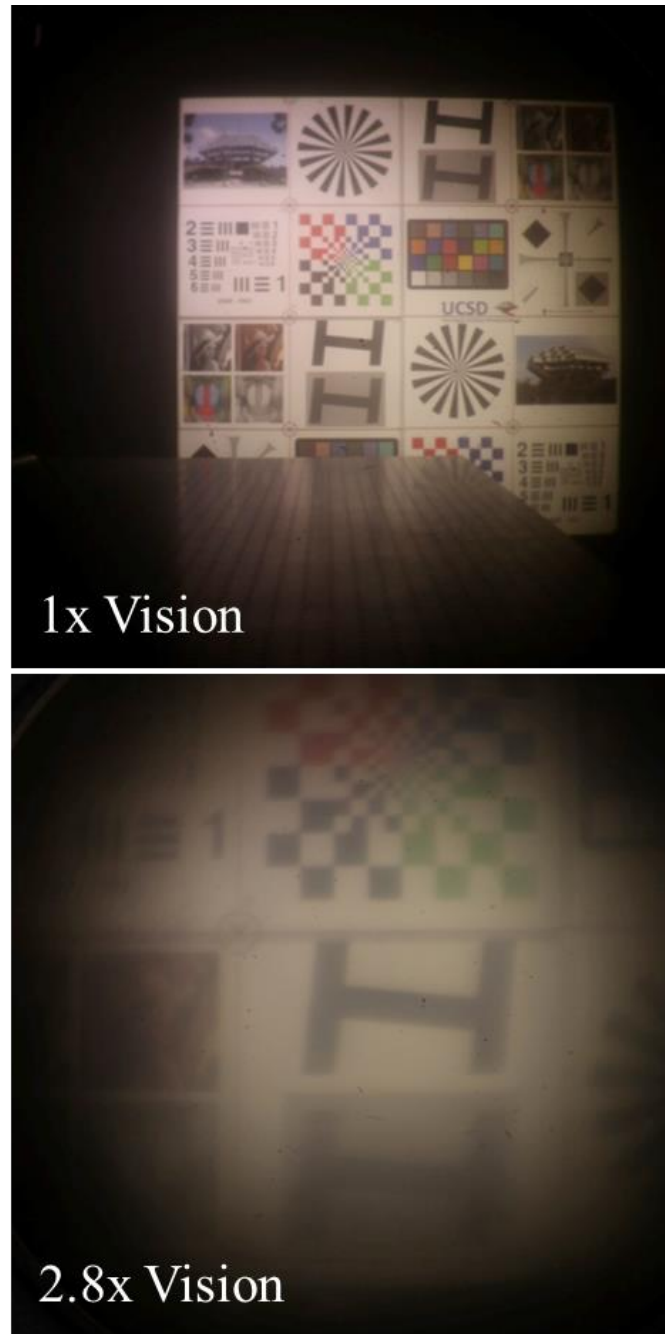
Figure 3-12: Image results of HFZ lens on eye model. (Top) 1x path and (Bottom) 2.8x path.
