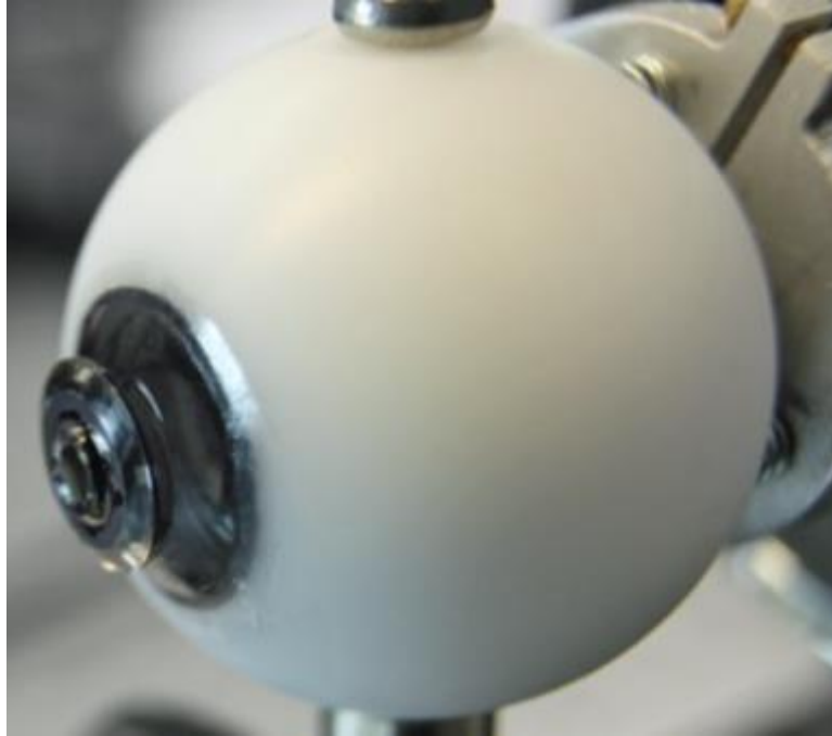
Figure 3-2: Generation-0 (not wearable) telescopic contact lens on an optomechanical eye model used for testing.
