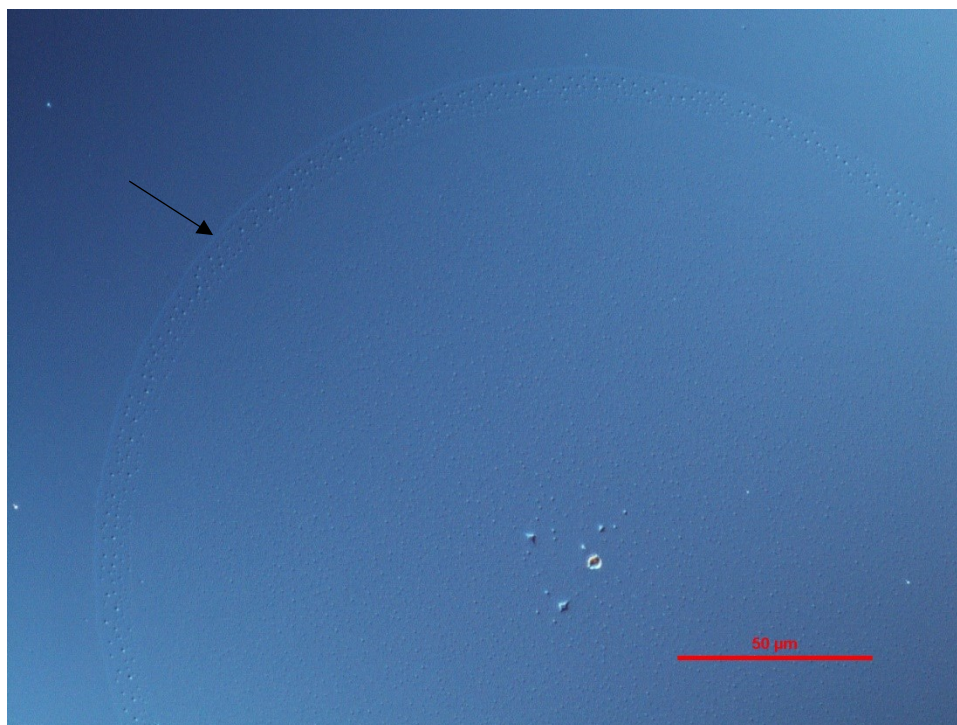
Figure 22. Optical micrograph of a different corrosion feature on 100Å SiN x over 5Å CrN x over Ag after 242 hr MFG exposure.
