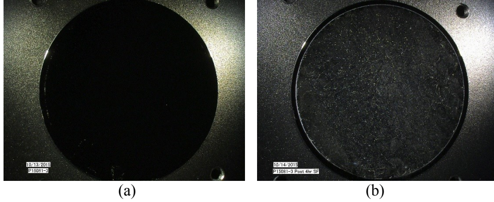
Figure 17. Dark field images of a mirror with 10Å of NiCrN x over Ag (a) before and (b) after 4 hr salt fog exposure.
