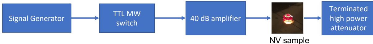
Figure 1.6: MW setup: A microwave signal generator (SRS SG386 or SG384) is used for both pulsed and continuous wave experiments. A MW switch (Minicircuits ZASWA-2-50DR) is used to shutter any spurious leakage in the MW channel. A high-power class A amplifier (Minicircuits ZHL-15W-422-S+) is used to amplify the MW prior to channeling the radiation to the NV sample. Downstream from the sample, a 50\Omega terminated high power attenuator (Minicircuits BW-N40W50+) is used to absorb the MW signal to prevent any reflection back to the sample.
