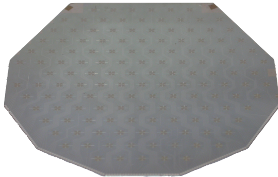
Figure 3.12: An EBEX array diced into its final decagonal shape for integration with the rest of the experiment
