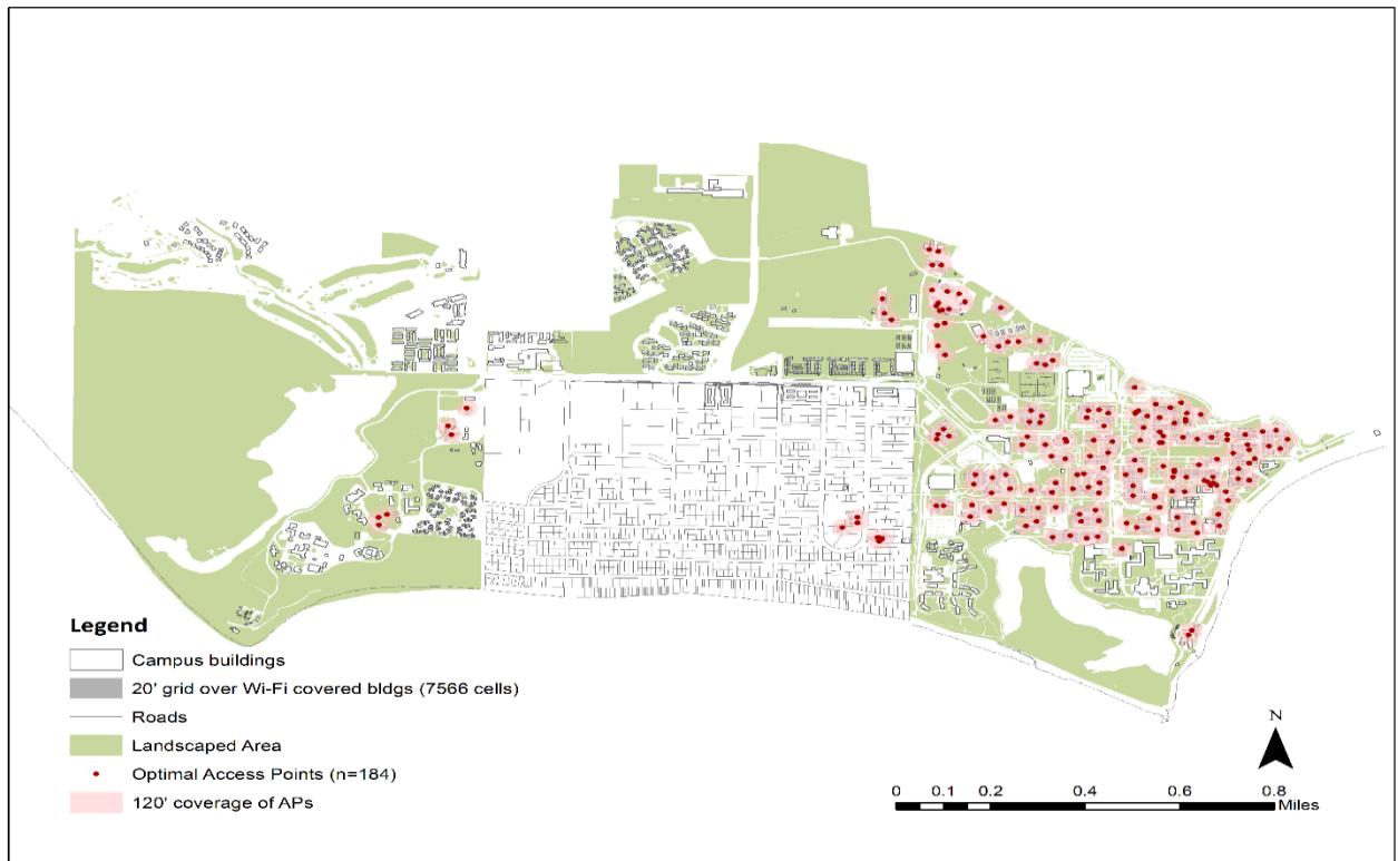
Figure 2: Optimal Wi-Fi configuration on UCSB campus (120 feet service distance)
