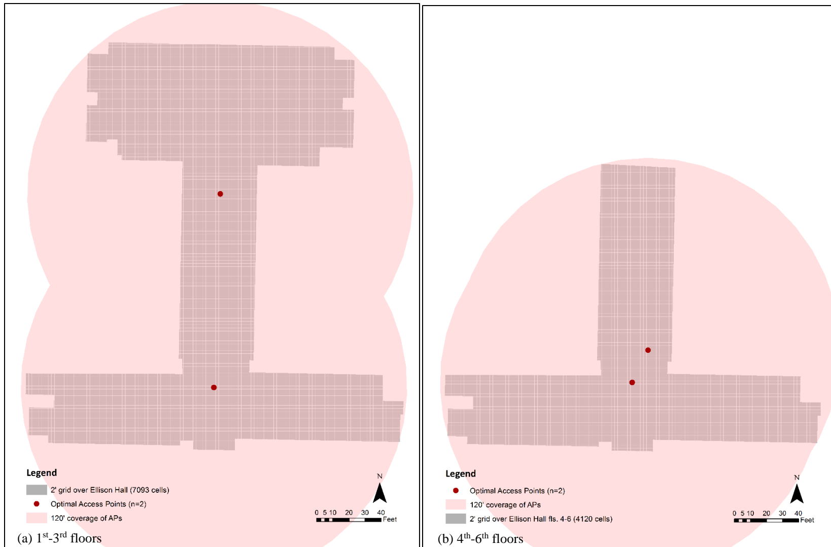
Figure 3: Optimal Wi-Fi configuration in Ellison Hall (120 feet service distance)
