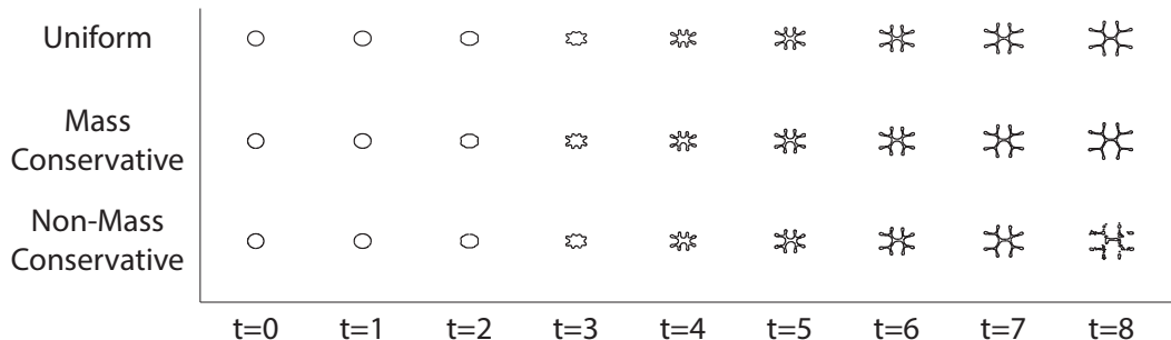
Figure 2.7: Evolution of tumor in 2D with \mathcal{P} = 0 , \mathcal{A} = 0 , \epsilon = 0.005 , D = 1 , \mathcal{X}_\sigma = 10 , and initial tumor surface as in Eq. (2.50). The \phi = 0.5 contours are based on uniform grid, mass conservative solver and non-mass conservative solver.
