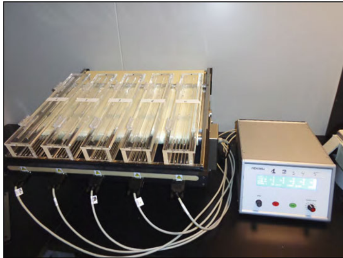
Fig. 1 Picture of the mouse treadmill apparatus. Five mice can be exercised simultaneously
