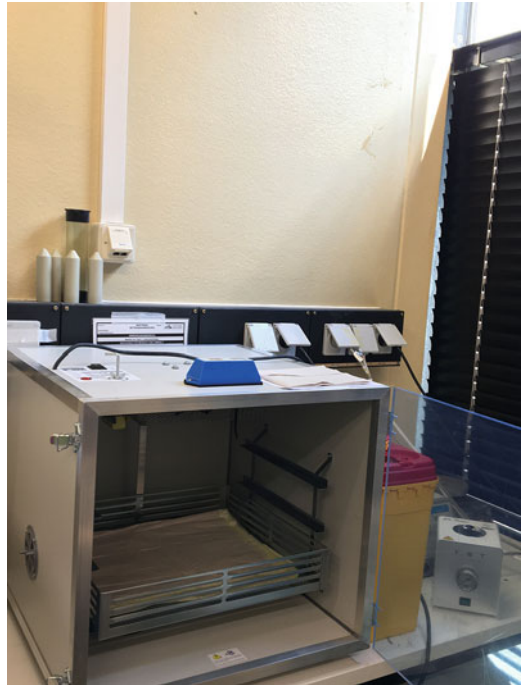
Fig. 3 Hatching incubator . Temperature and humidity can be regulated and feedback controlled. Due to constant ventilation, temperature is evenly distributed within the incubator
