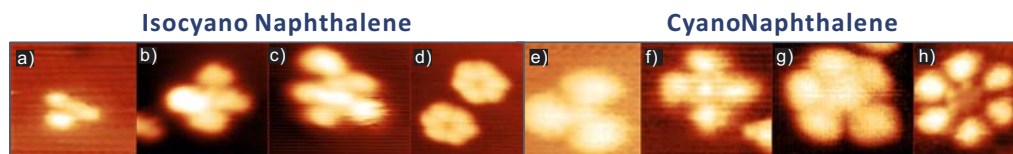
Figure 6.2: The left four images a)-d) are 3-6 fold coordination patterns for isocyano compounds, the right four images e)-f) are the same patterns but for cyano compounds
