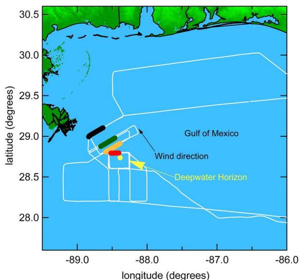
**Figure 1.** Map of the WP-3D flight track (white line) over the Gulf of Mexico on 10 June 2010. The yellow circle marks the location of the DWH oil platform. The aircraft sampled plumes in the atmospheric MBL at four distances downwind from DWH indicated by the thick bars: 10 km (red), 20 km (orange), 30 km (green), and 50 km (black).
