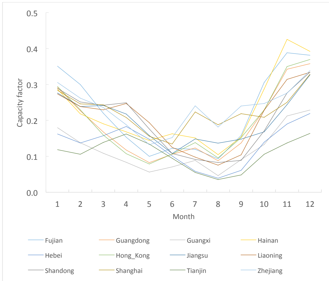
Figure 2-4 Monthly average offshore wind capacity factor 2001-2010
