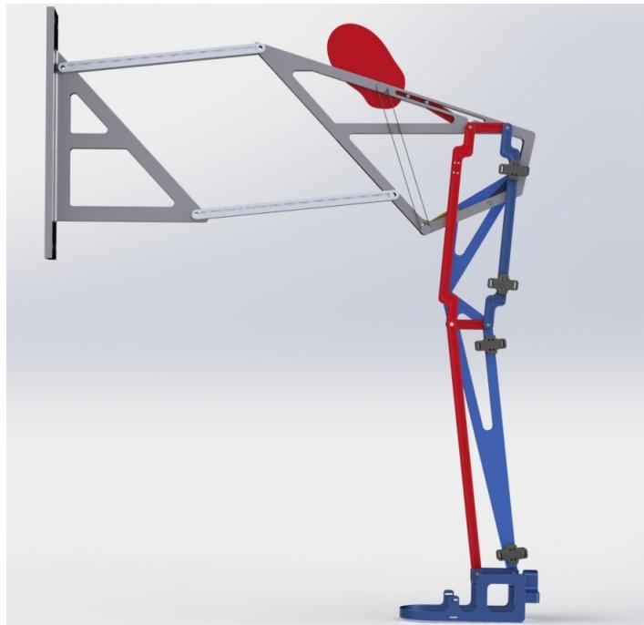
Figure 8.6: The parallelogram mechanism attaches to the six-bar linkage in order to control the foot orientation angle.
