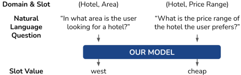
Figure 3.3. Based on a dialog history, a natural language questions are provided to our model to query a user’s requirements and preferences (dialog state). We construct questions to resemble colloquial human speech, in contrast to approaches that use templated questions [120].
