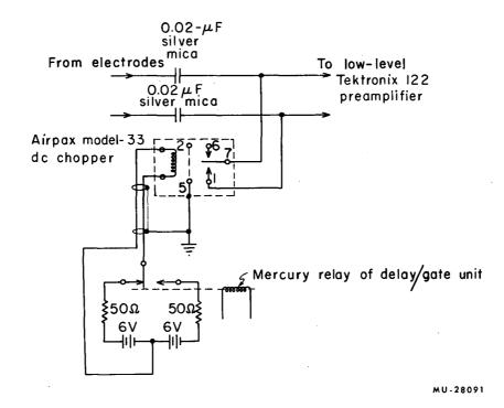
Fig. 7. Gating switch on amplifier input.
