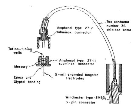
Fig. 5. Mounted or chronic-implant-type electrode showing cable connector (scale  $\approx 2X$ ).
