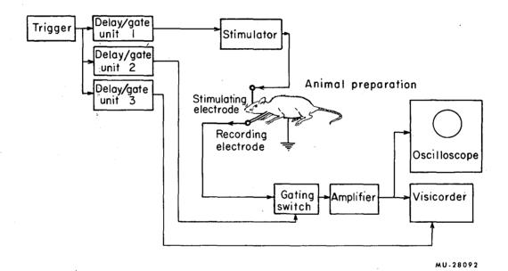
Fig. 1. Diagram of system.
