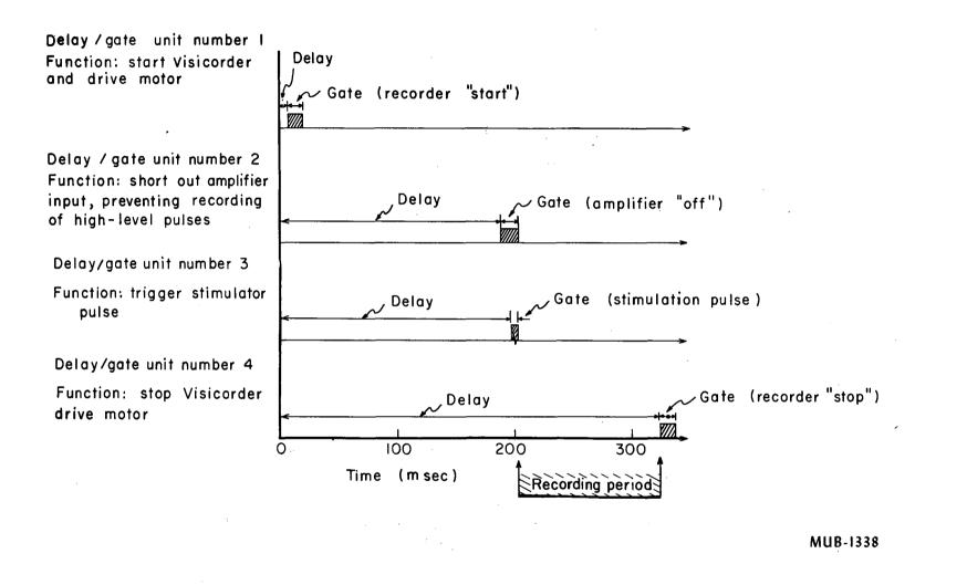
Fig. 10. Use of time-base units to synchronize stimulation and recording. At time t = 0, the trigger pulse activates all delay/gate units.
