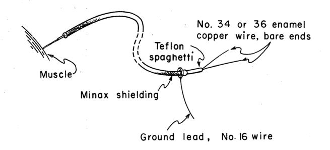
Fig. 2. Electromyogram electrodes.
