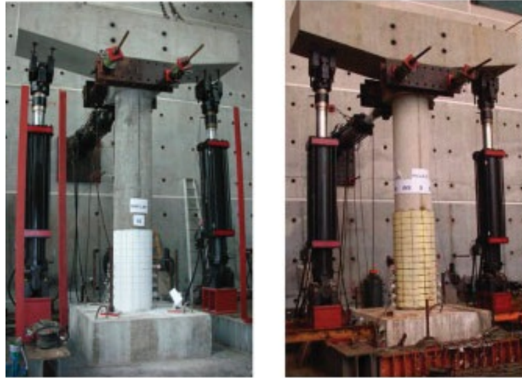
Figure 2.13 Constructed bridge piers under two different conditions: fixed-base (left) and rocking-base (right) (from Hung et al. 2011).
