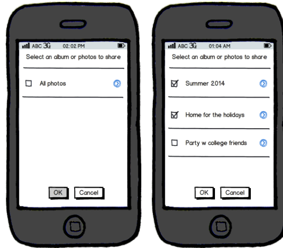
(a) The application wants to read the user’s photos, so it opens this chooser. (b) After clicking on the right arrow, the user selects two albums.
