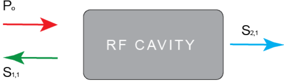
Figure 2.7: S-parameters for transmission and reflection power measurements schematic.
