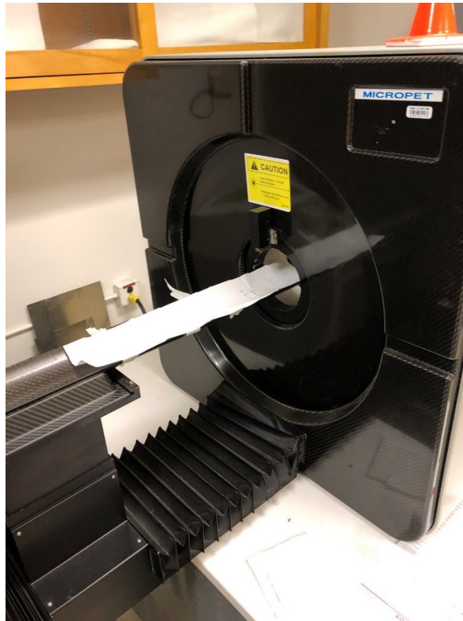
Figure A.1: Sarah , the Concorde MicroPET R4 used for the preclinical studies in this dissertation.
