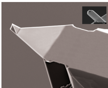
Figure 3.23: SEM images of two different probes used for dissolution experiments. The large image is the Arrow UHF probe. The small probe in the inset, approximately to scale, is the USC f1.2 k0.15 probe, which is preferable to the Arrow UHF for studying soft polymers due to its lower stiffness, but presents challenges for the feedback laser due to its reduced size.
