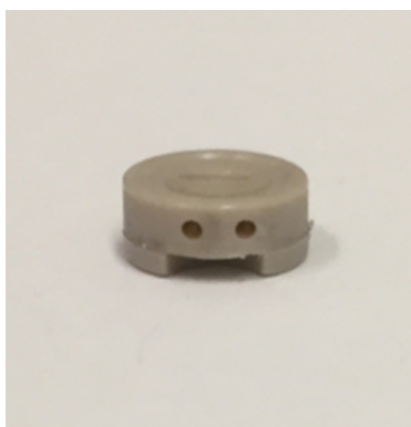
Figure 3.22: Current flow cell. Excess mass has been removed to push resonant frequency of the piezo-flow cell system as high as possible.
