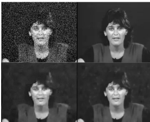
Figure 4.2: Frame 5 of the Miss America sequence: Visual comparison of a frame corrupted by AWGN of \sigma = 30 (top left), the original frame (top right), the VBM3D result (bottom left) and the output of the proposed method (bottom right)
