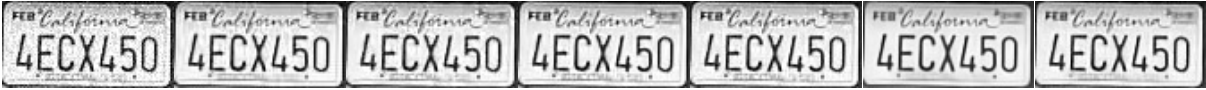
(b) Noisy ( \sigma = \frac{20}{255} ) (c) BM3D (25.77, 0.9497) (d) EPLL (25.51, 0.9508) (e) tar-EPLL (26.84, 0.9624) (f) tar-EPLL3 (26.47, 0.9586) (g) TID (25.37, 0.9525) (h) FED (26.47, 0.9541)
