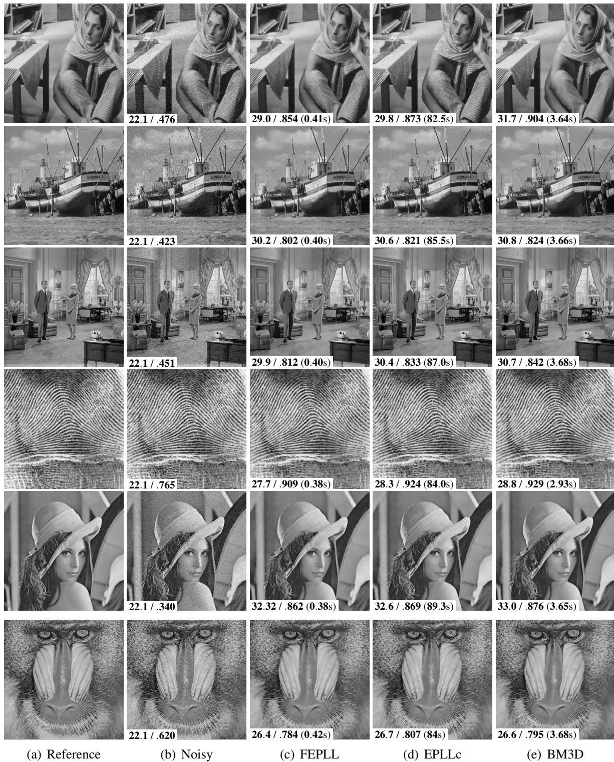
Figure A.6: Denoising results where \sigma=20 obtained on five standard images, from top to bottom: Barbara, Boat, Couple, Fingerprint, Lena and Mandrill.
