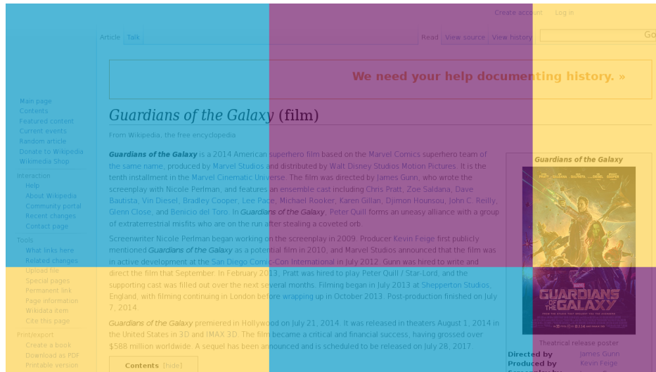
Figure 2.3: Parallel painting on a Wikipedia page using 3 threads. Different colors indicate that painting was performed by a different thread
