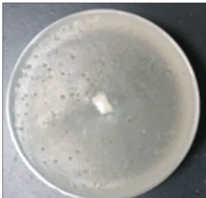
Figure 2. Enamel chip embedded for microhardness testing.
