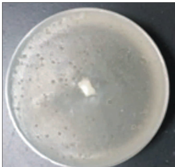
Figure 2. Enamel chip embedded for microhardness testing.
