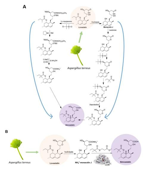
**Figure 1.** Synthetic methods for cholesterol-lowering agent simvastatin. (A) Traditional chemical syntheses. (B) Chemo-enzymatic synthesis with LovD mutants.
