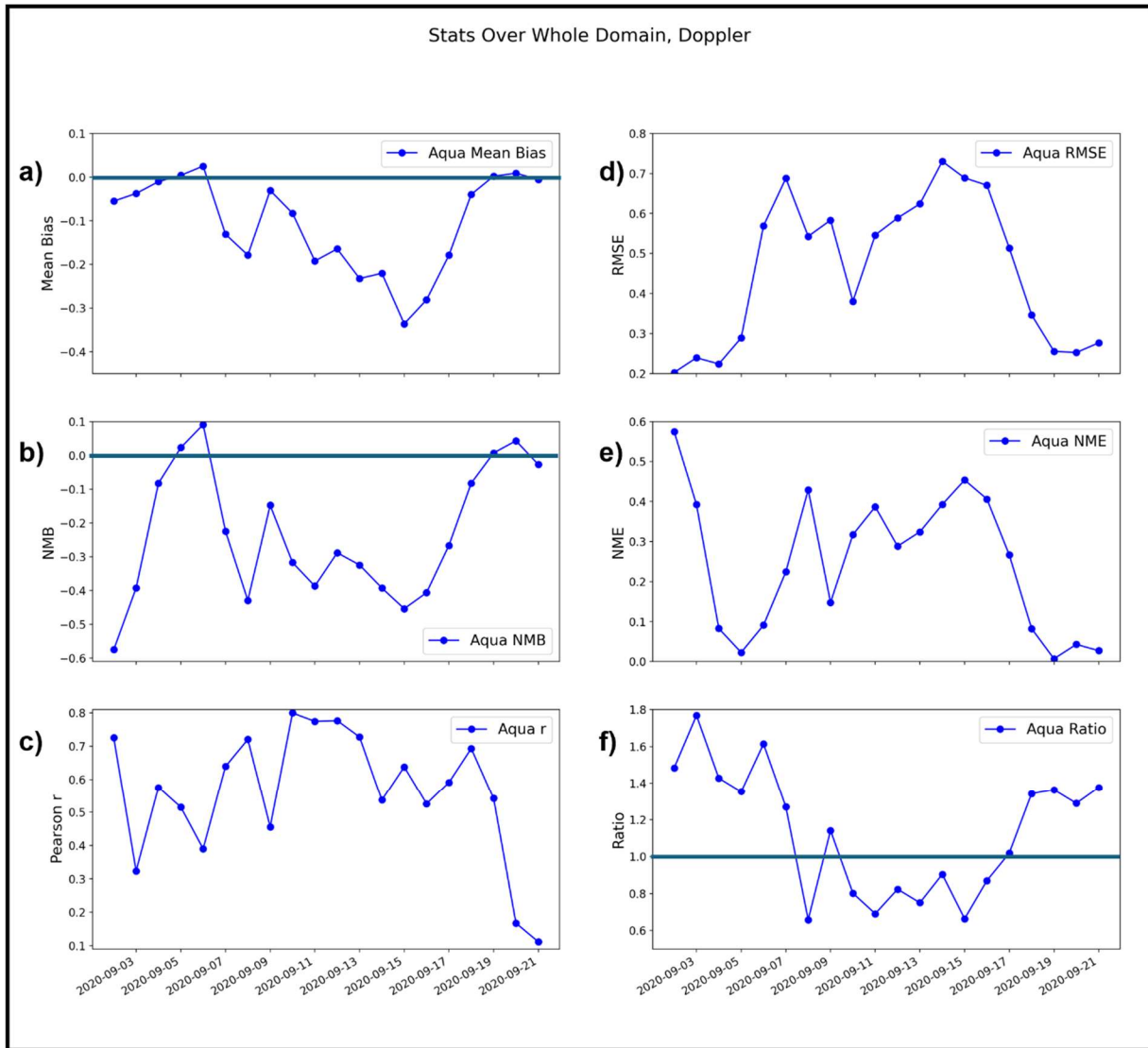
Figure 4.5: Time series of whole-domain AOD statistics comparing the Doppler WRF-Chem run and AOD from the MODIS instrument on Aqua, using the MAIAC algorithm. Plots show (a) mean bias against observations; (b) normalized mean bias; (c) Pearson r correlation coefficient; (d) root-mean-squared error; (e) normalized mean error; (f) ratio of modeled to observed AOD value. Horizontal lines are superimposed at the level of unity—a bias of zero, or a ratio of 1 between model and observations.
