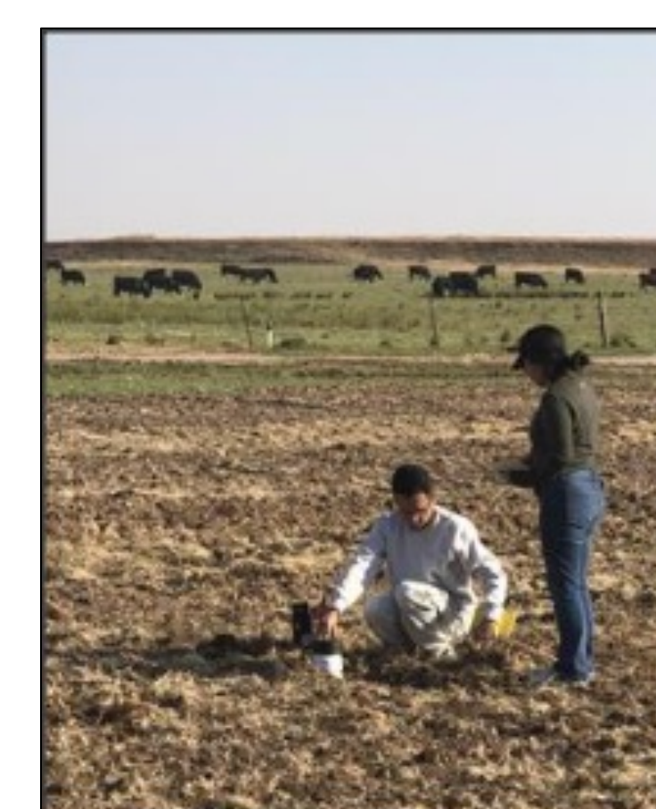
Students collecting CO 2 efflux manually using low-cost flux chamber
