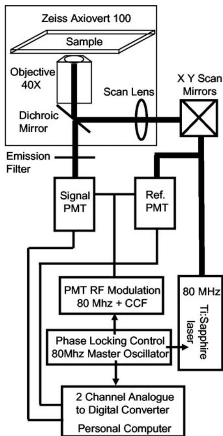
FIGURE 2 Experimental diagram of the two-photon fluorescence lifetime imaging instrument.
