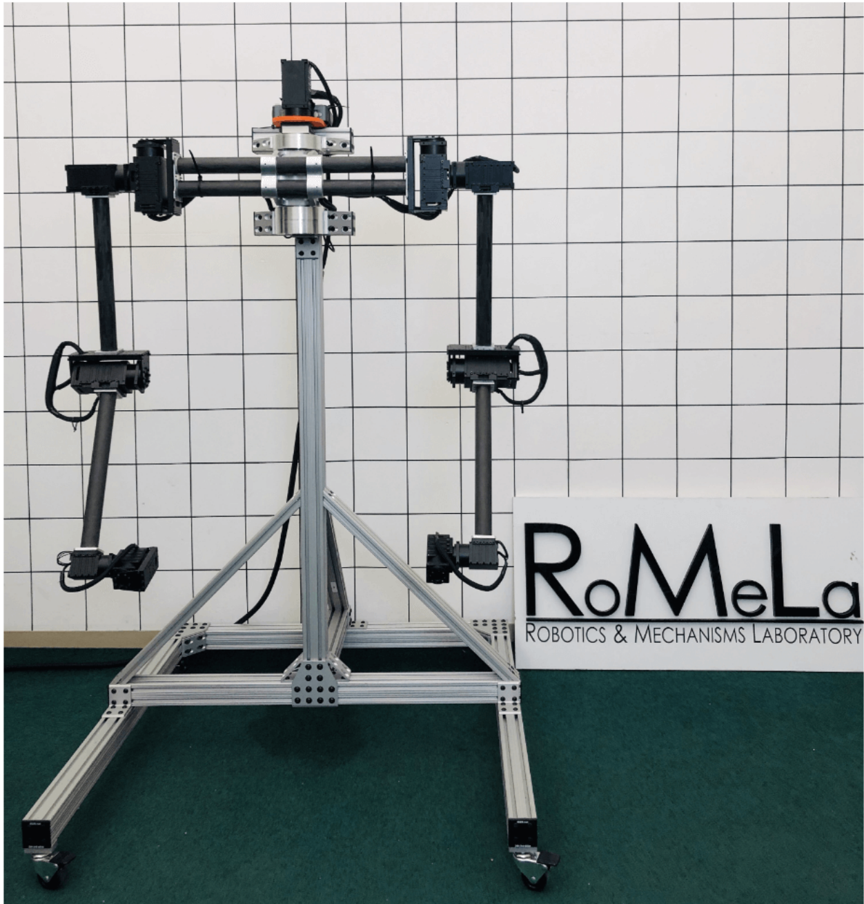
Figure 2.4: Prototype of the dual-arm manipulator.
