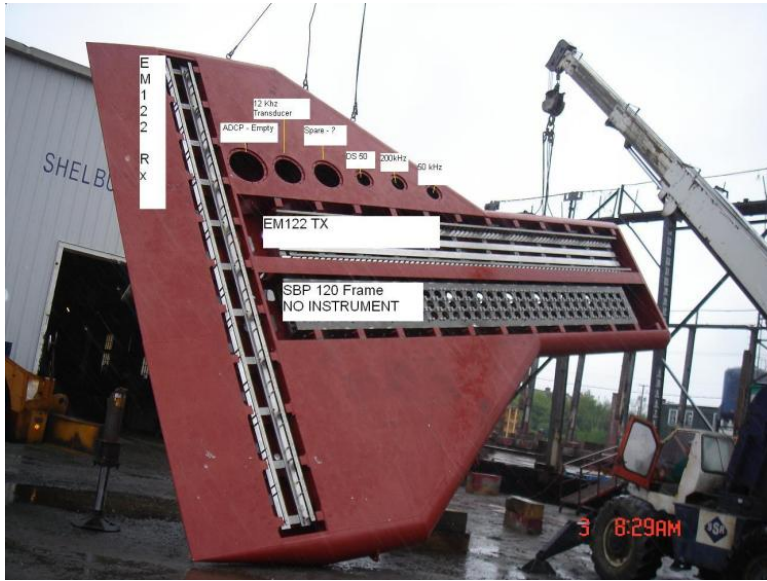
Figure 2: Gondola containing a 7 m long array of transducers (EM122 TX) that are oriented parallel to the keel of the ship and a 7 m long array of hydrophones (EM122 RX) perpendicular to the keel. This system is a Kongsberg EM122 multibeam sonar being mounted on the hull of the RV Langseth. (Photo credit, John Greene, Texas A&M).
