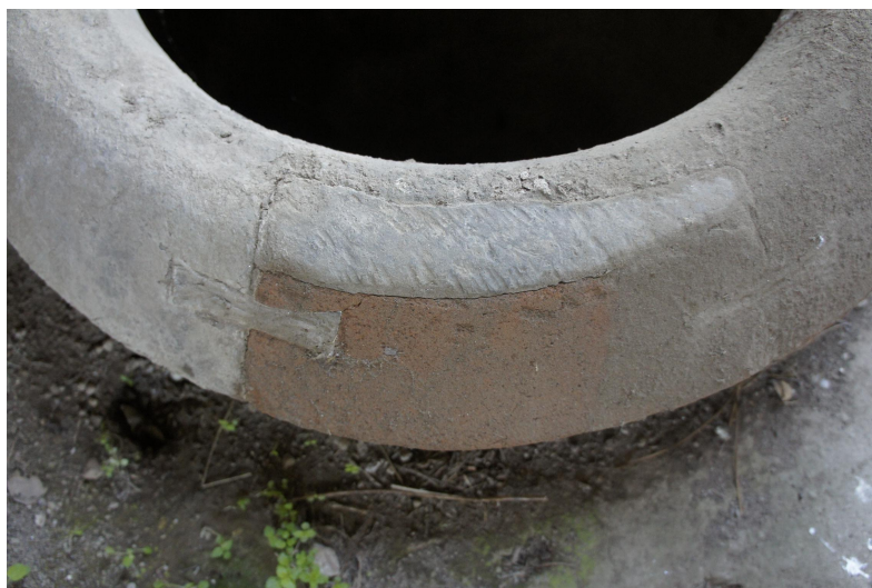
Fig. 4.27. Large lead fill (and lead double dovetail) on dolium rim (II.5.5 no. 10), Pompeii.
