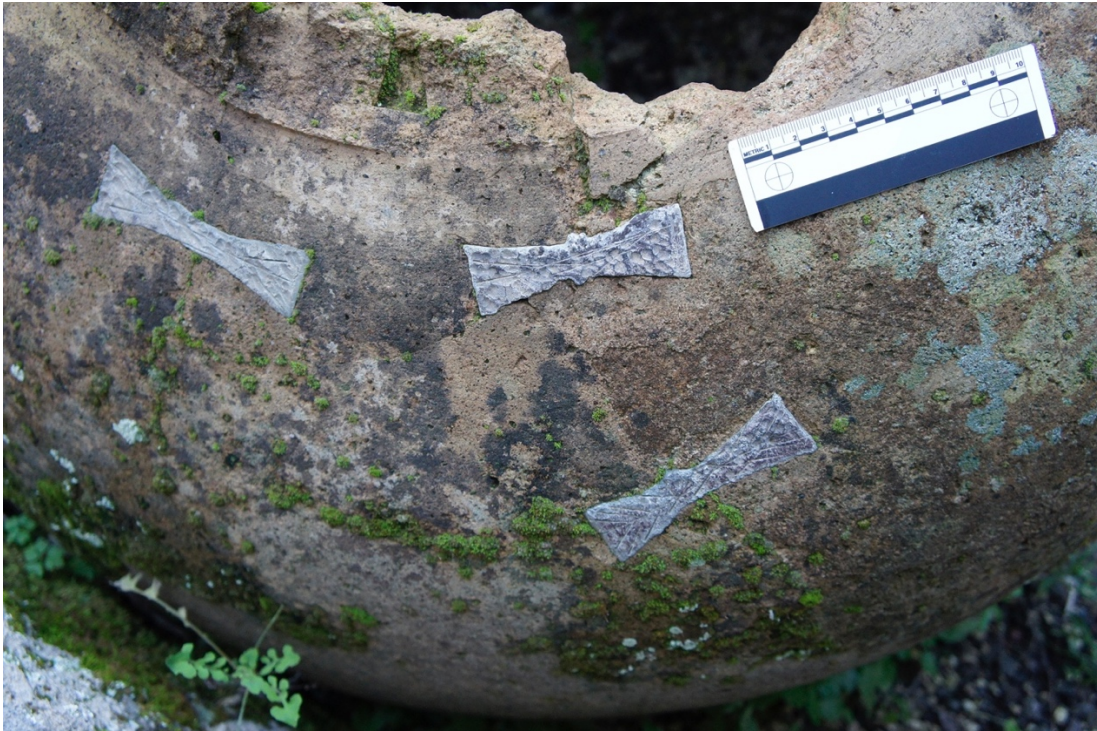
Fig. 4.34. Dolium repaired during production with double dovetails (I.21.2 n. 1), Pompeii.
