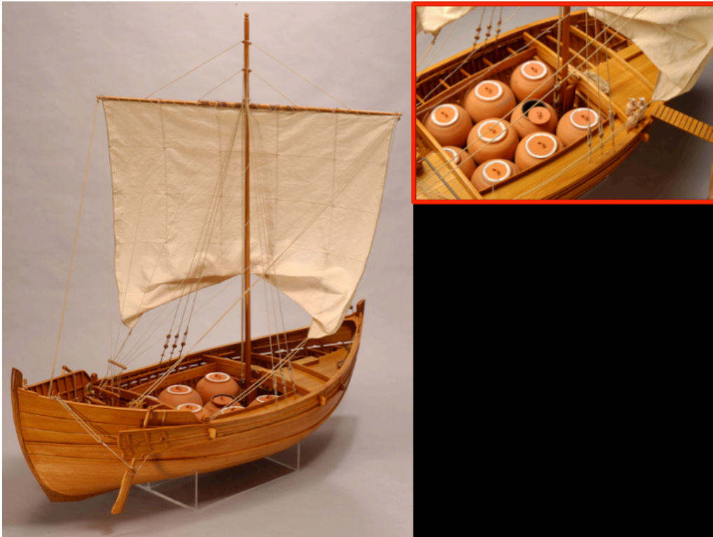
Fig. 3.3. Reconstructed model of specialized wine dolium ships, by the Centre National de la Recherche Scientifique, Centre Camille Jullian.
