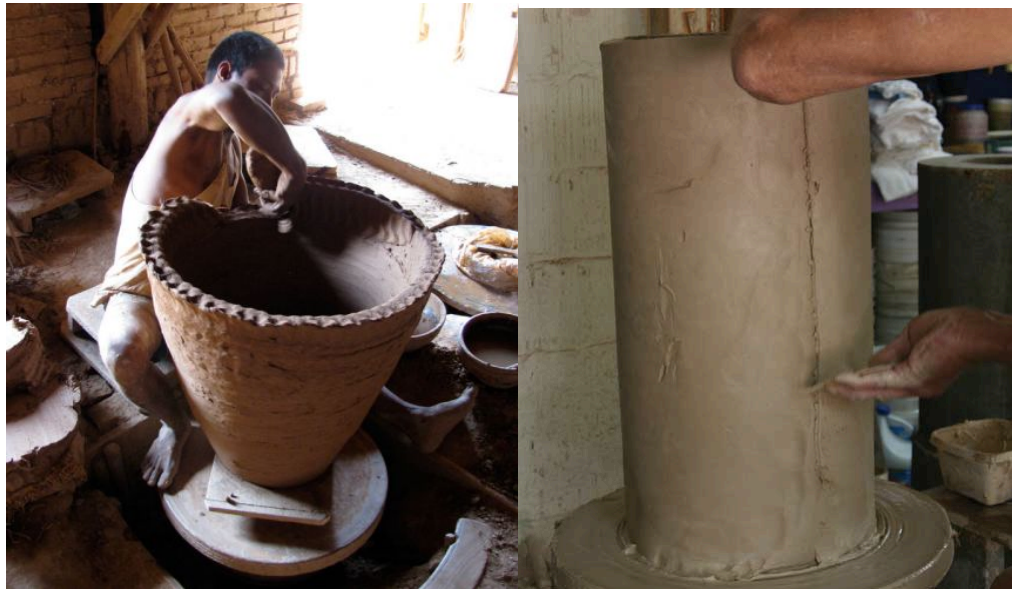
Fig. 12. (L) Contemporary Burmese potter coil-building a traditional storage jar. Fig. 13 (R) Contemporary potter slab-building a vase.
