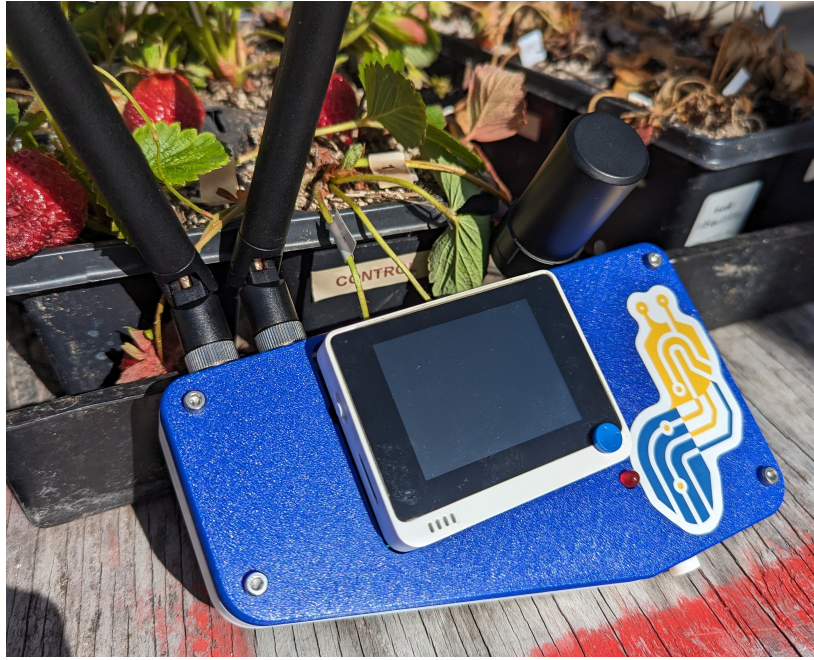
Figure 3.10: Image of the Handheld Clicker. The two antennas on the left are the UHF antennas and the one on the right is the RTK antenna. The screen in the middle is the Wio terminal.
