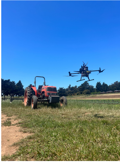
Figure 2.1: Image of our quad-copter drone (a DJI Matrice M300) with heavy lift capabilities hovering in the field.
