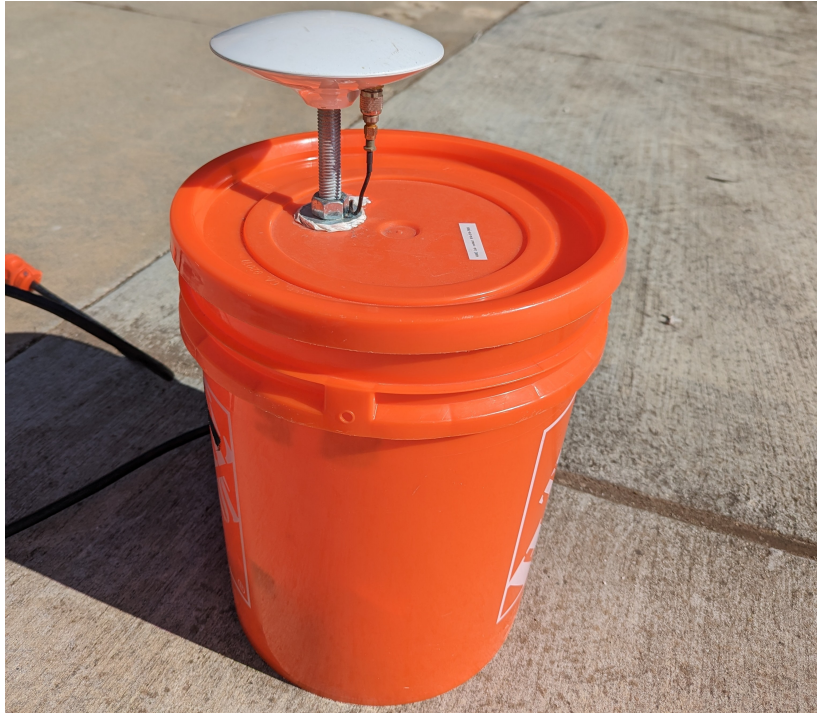
Figure 3.9: Image of our RTK base station. The lid remains removable even with the RTK antenna protruding from the top.
