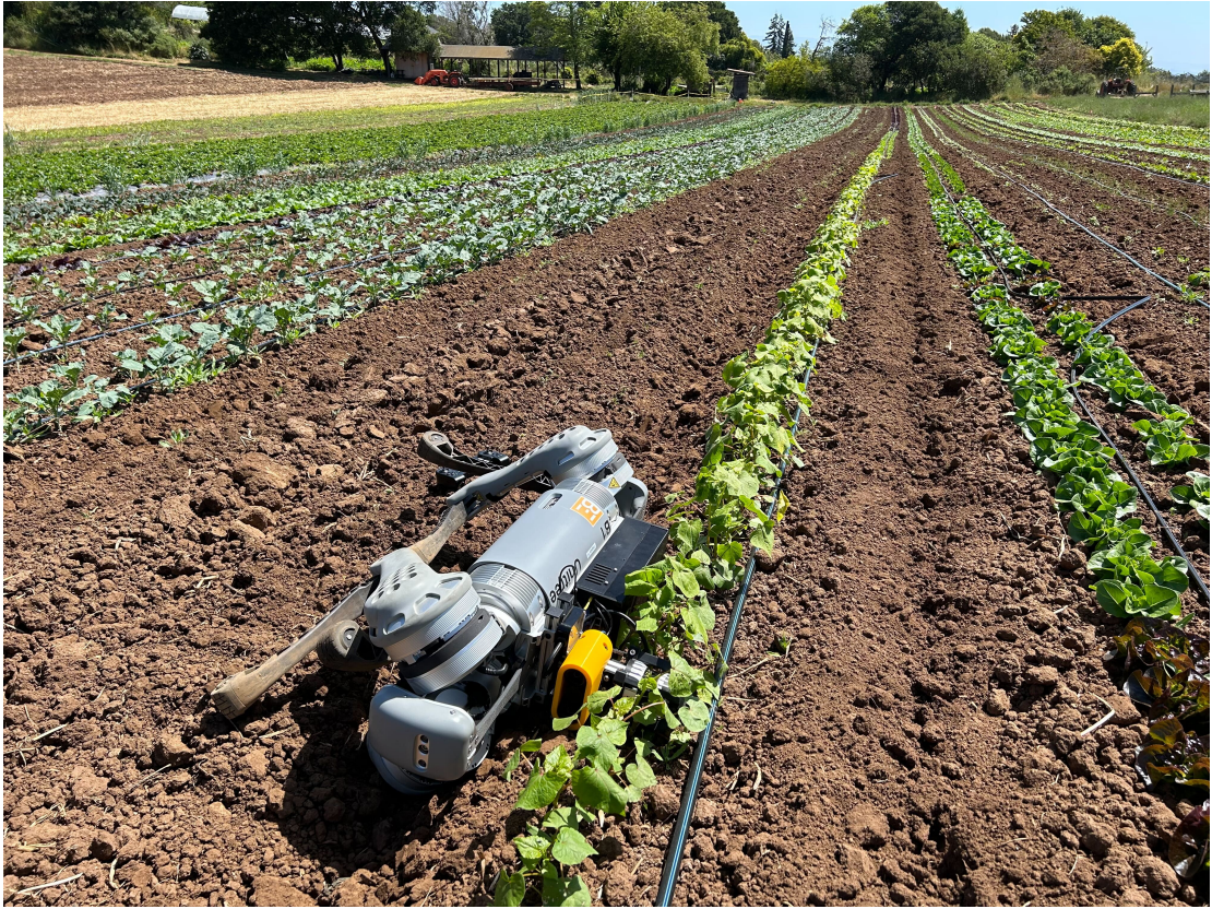
Figure 2.3: Photo of a Unitree B1 quadruped robot fallen over after attempting to navigate through soft dirt. Terrestrial based robots can struggle to navigate through farms due to restrictions such as dirt texture, furrow spacing, and a high risk of damaging crops.
