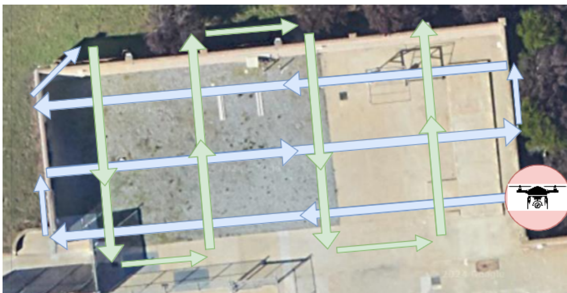
Figure 4.2: Polygon flights visualization. The drone begins at the red circle and flies the first horizontal polygon flight in blue. After finishing that orientation, it proceeds to fly the vertical polygon in green. AprilTags are randomly placed within this grid.
