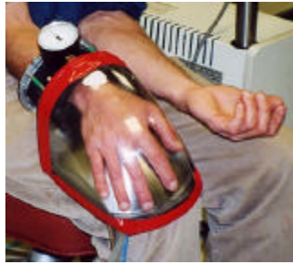
Figure 5.56 Low pressure device to help the heat loss from the hand (Department of Biological Science, Stanford University, 2002)
