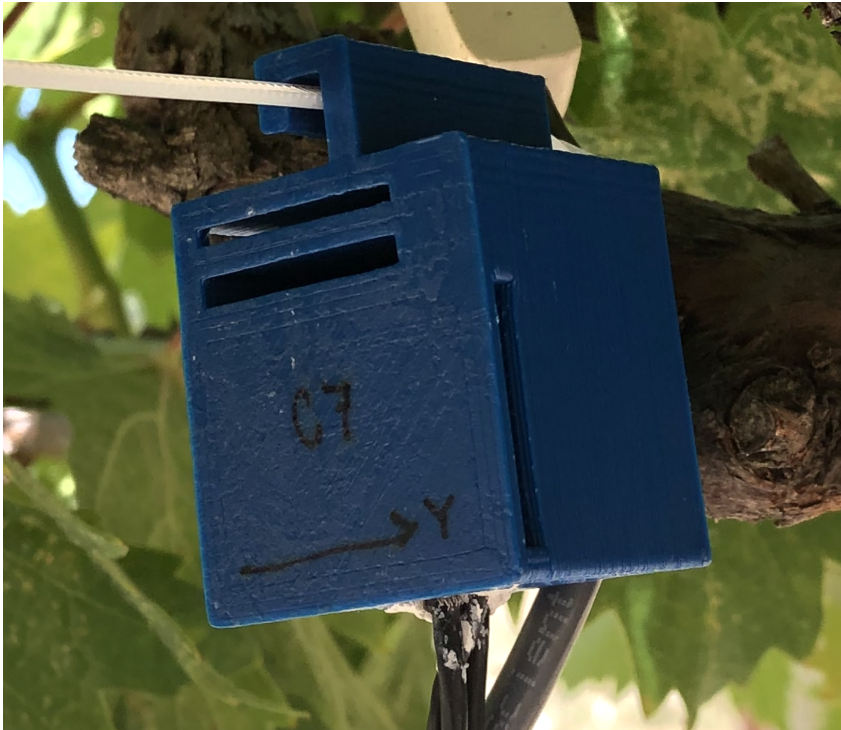
Figure 3.1: An example of a 3D printed low-cost Cube sensor deployed in the field.
