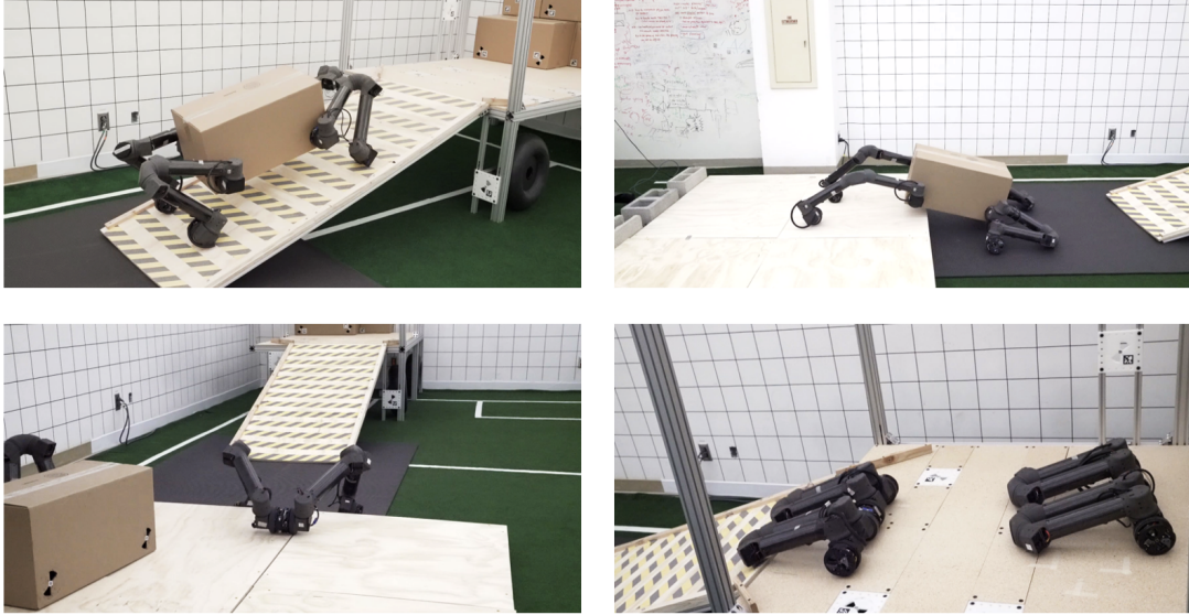
Figure 6.1: Frames taken from the LIMMS demonstration moving a box out of the truck and delivering it to a location and returning. ( Top Left ) shows LIMMS quadruped mode rolling down the ramp. ( Top Right ) depicts a workaround that had to be made to compensate for the extra motors to get LIMMS to climb a step. ( Bottom Left ) illustrates a three wheeled mode used to return when overcoming obstacles. ( Bottom Right ) shows an aligned four wheel mode used to traverse flat surfaces to return.
