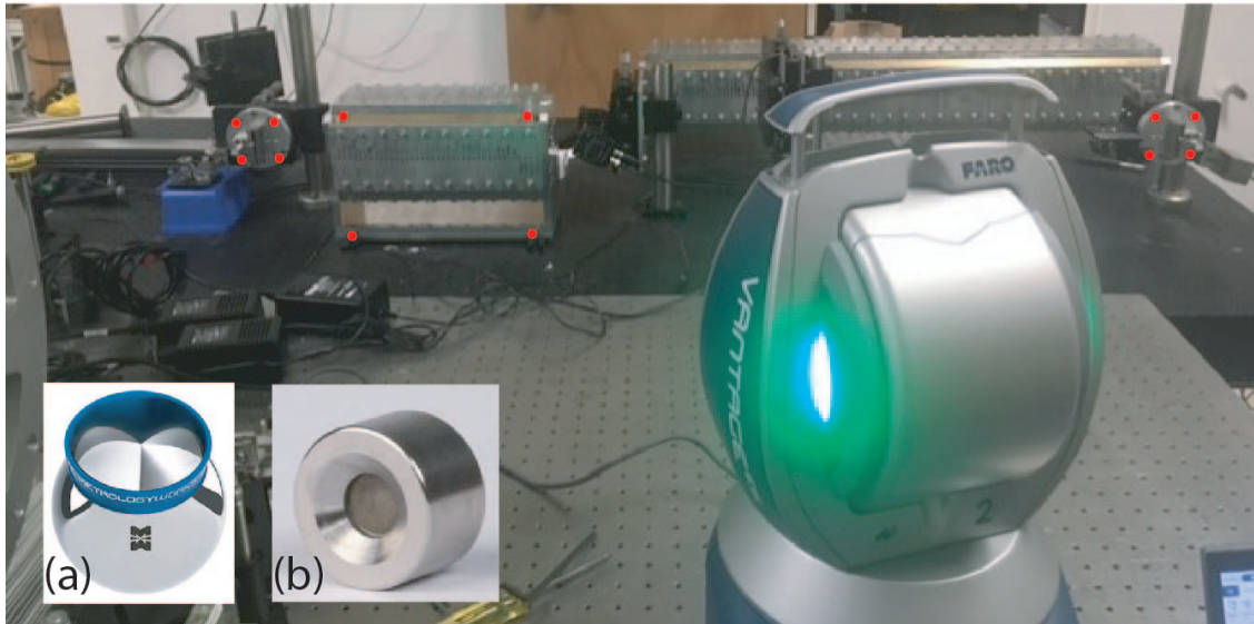
Figure 3.21: Fiducialization of the FASTGREENS prebuncher. The laser-tracker accurately measures the distance to the retroreflector (a) when placed in each of the fiducial cups (b). Locations of fiducial cups are marked in red.
