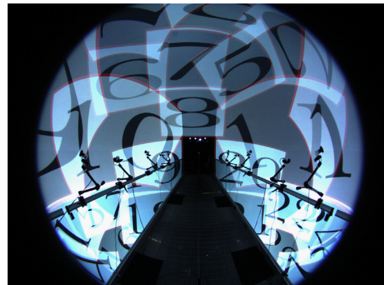
Fig. 8. Fisheye photograph from the bridge showing most of the 26 overlapping projection areas and calibration cameras mounted to the bridge railing.
