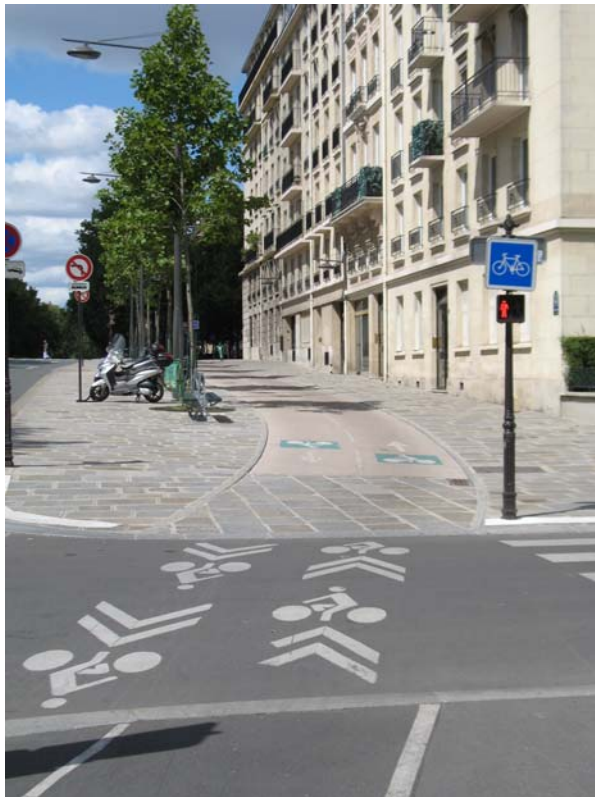
Figure 4. Representative example of a sharrow symbol (This particular example comes from Paris)
