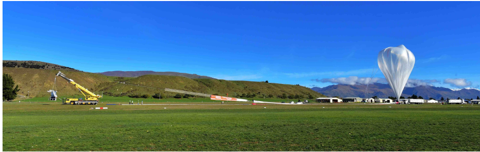
Figure 5.1: Photograph after the Super Pressure balloon has been inflated and immediately before launch on May 17th, 2016, in Wanaka, New Zealand. COSI , hanging from the launch vehicle, is visible on the left side of the photograph, the orange parachute is in the middle, and the balloon is on the right. Only partially inflated on the ground, once the balloon reaches float altitudes it becomes fully expanded with a diameter of over 100 m. The Wanaka Airport can be seen in the background, which includes the hangar within which all integration occurred.
