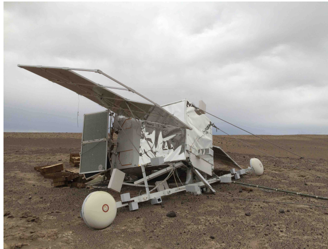
Figure 5.3: The instrument was located in the desert north of Arequipa, Peru, on July 7, 2016, just 5 days after termination. Although the gondola frame was bent and the antenna booms and some solar panels were destroyed, all of the COSI instrument systems have been tested after flight and are operational.
