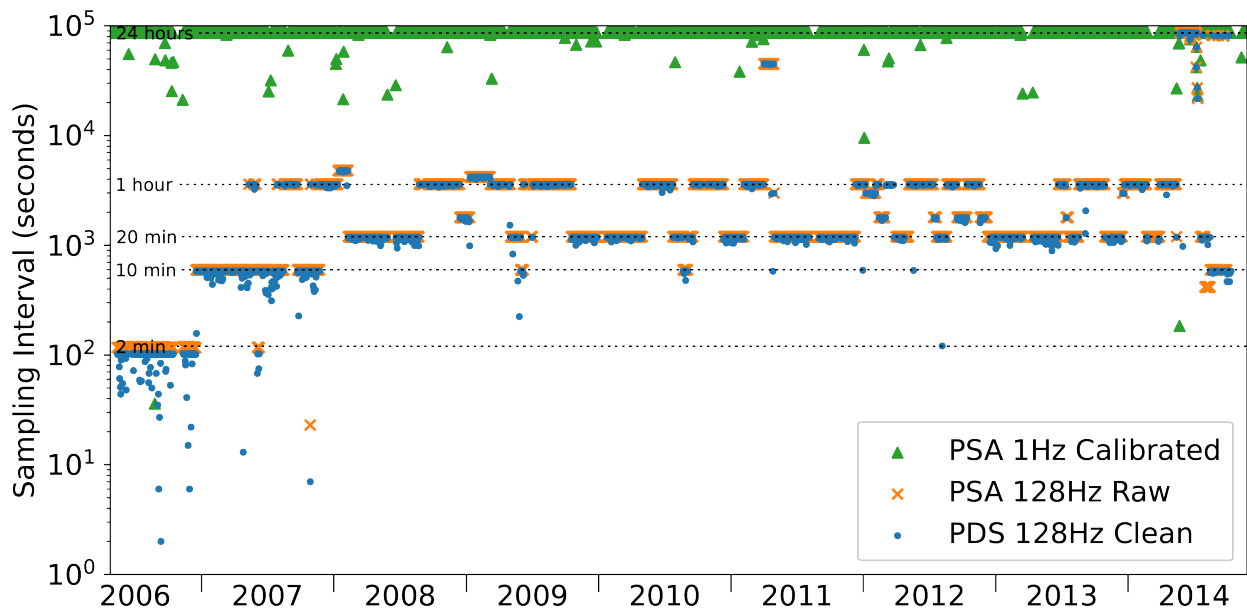
Figure 2.4: Sampling intervals for each available orbit in the three data sets referenced herein. Each value is the difference between the first and the last times of that particular orbit.
