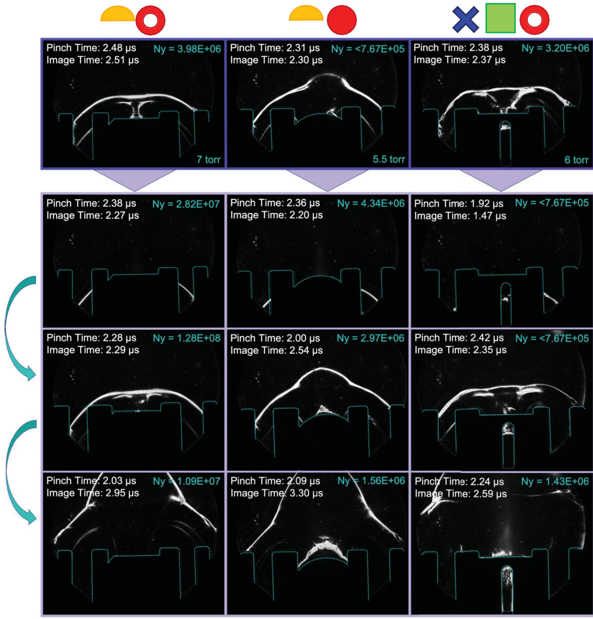
Figure 3-3. Schlieren images of well-timed pinches for each anode as well as corresponding time evolution images. The anode and cathode rods are outlined to improve visibility. The ideal pinch is one that has minimal instabilities and a uniform and dense column is produced at the tip of the anode. The hemispherical solid anode was not able to properly support the production of a stable pinch. The corresponding pressures to each of these well timed pinch shots are shown at the bottom right of each image. For the time evolution images, each of these were different shots taken at the same pressure of 5 torr. Their corresponding neutron yields are found on the top right of each image.
