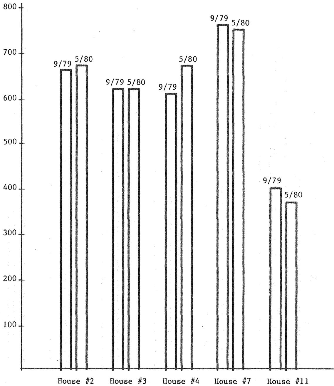
Figure 1- Cell #1 pre and post-retrofit effective leakage areas (cm<sup>2</sup>).
