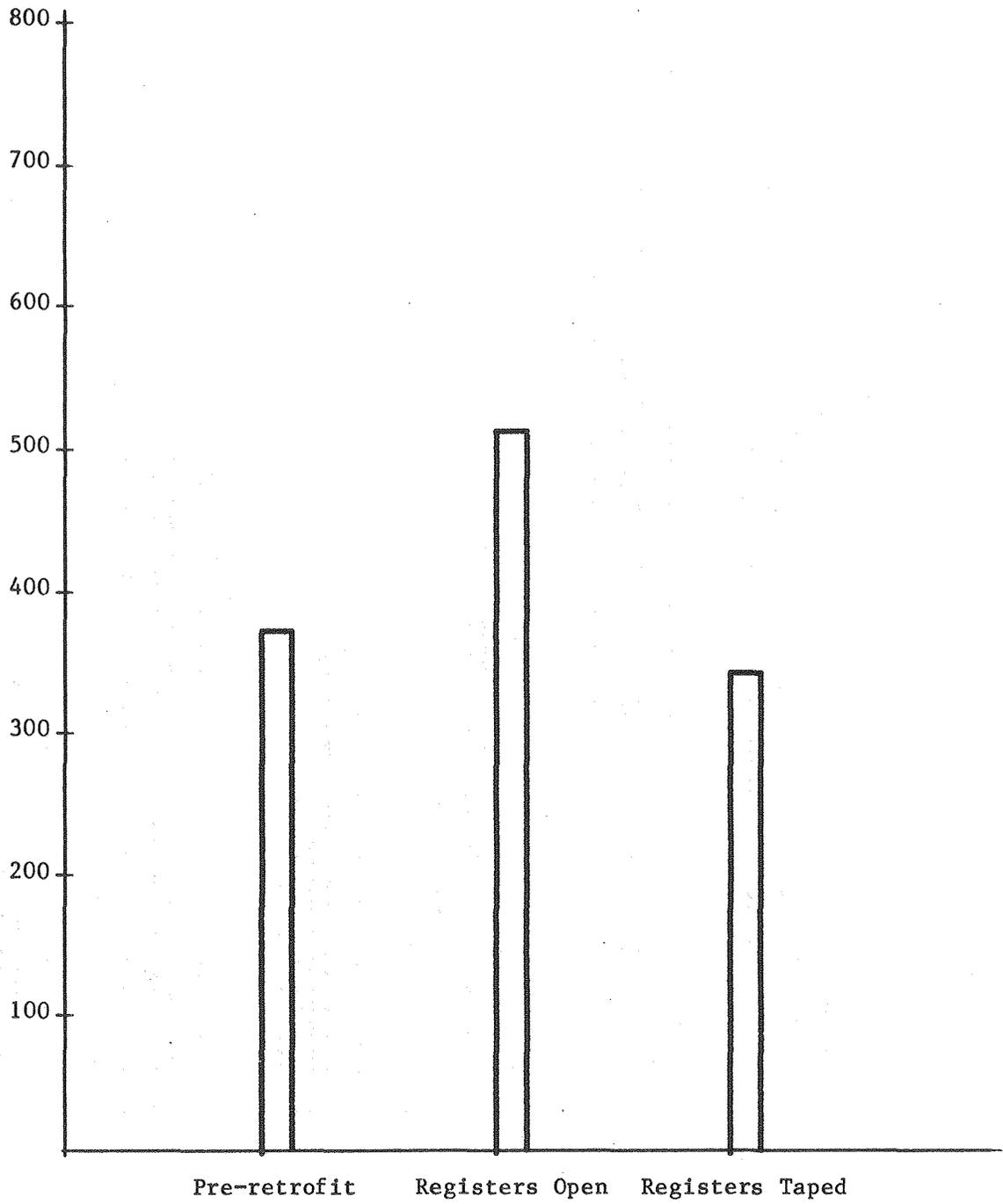
Figure 4- House #19 effective leakage areas (cm<sup>2</sup>).
