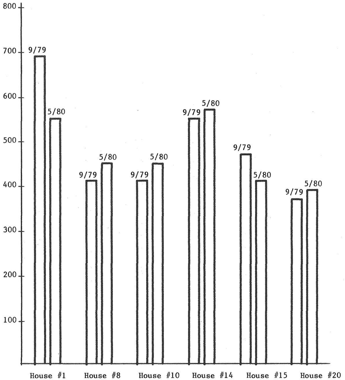
Figure 2- Cell #2 pre and post retrofit effective leakage areas (cm<sup>2</sup>).
