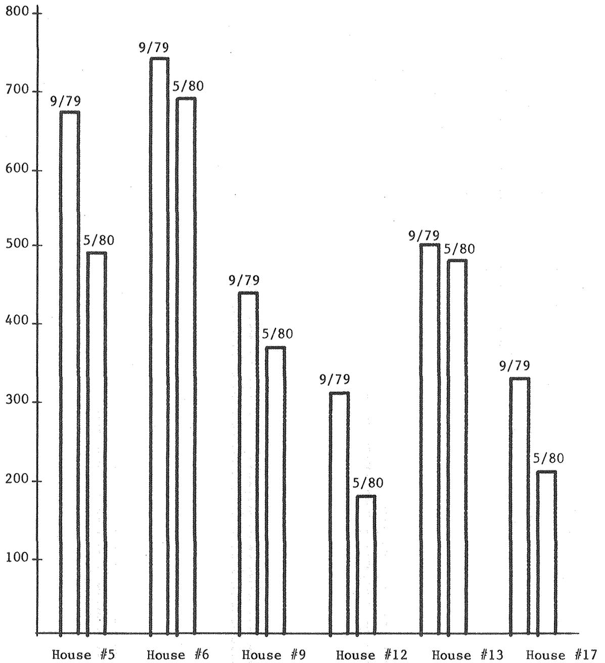
Figure 3- Cell #3 pre and post-retrofit effective leakage areas (cm<sup>2</sup>).
