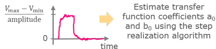
Figure 7.3: Procedure used to determine the heater power to contact sensor transfer function as a function of DC level in heater power.
