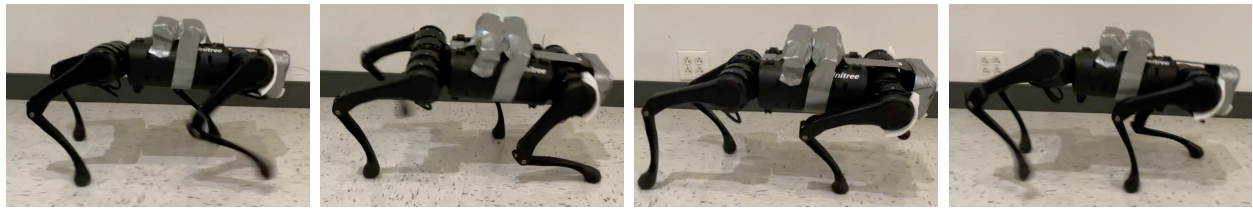
Figure B.1: Key frames of the walking gait, trotting gait and bouncing (galloping) gait. Red dots indicate foot contacts.
