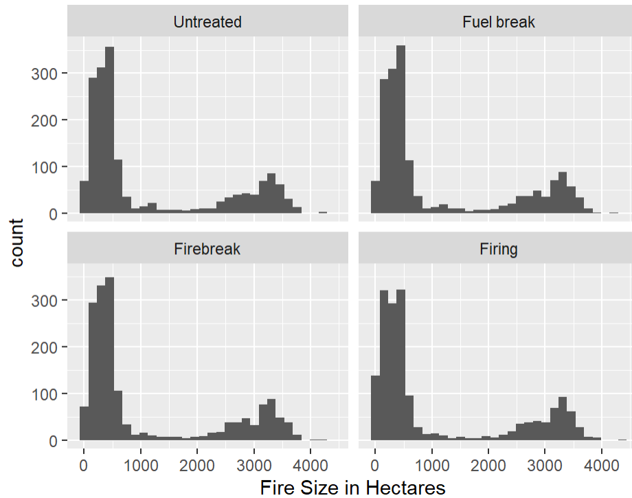
Supplementary Figure 2: Fire size distribution of the Single Segment Fuel Break Limestone Ridge Landscape. Generally, fire sizes shift left as leverage intensity increases, while the histogram shape remains mostly unchanged.
