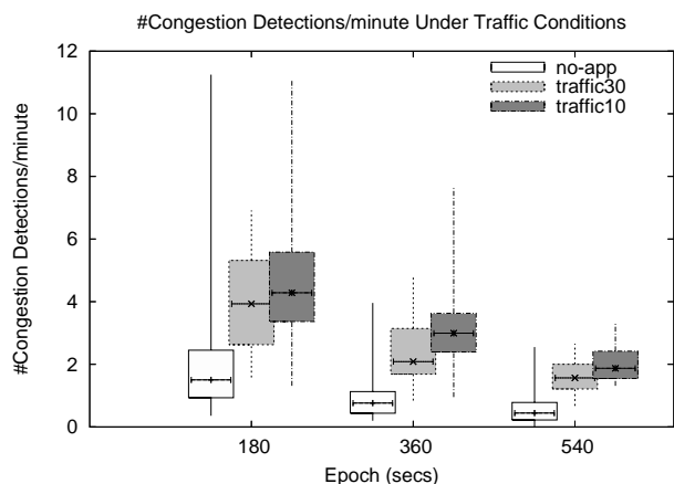
Figure 10: Number of collision detections vs. epoch. Congestion root causes increase with traffic, making collision notifications a good indicator for congestion detection.
