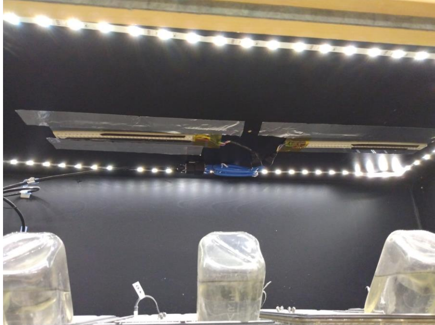
Figure 1. LED light strips for generating Light/Dark (LD) cycles in light-tight chambers. The LD cycle was generated via LED light strips that were placed along the perimeter of the environmental control chambers and were controlled by an external timer. The LD cycle consisted of 12 hours of light (250lx; 3000K) and 12 hours of darkness. K=Kelvin; lx=Lux
